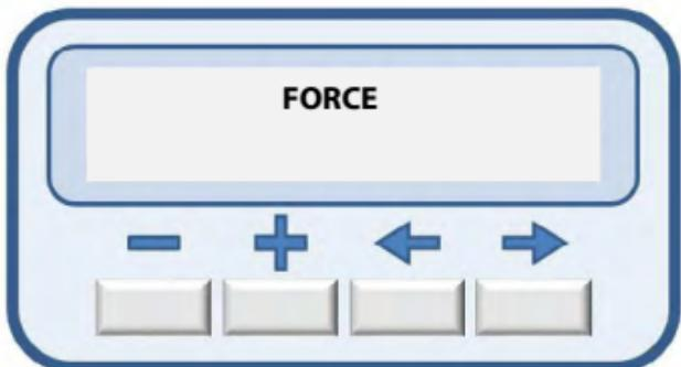
Power is shipped from the factory at the maximum level. To decrease it, just press the (-) key until the desired level, and to increase it, just press the (+) key.
