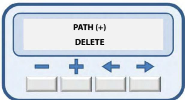
To delete the memorized path, press and release the (+) key. To record the path again, press and release the (+) key one more time.
