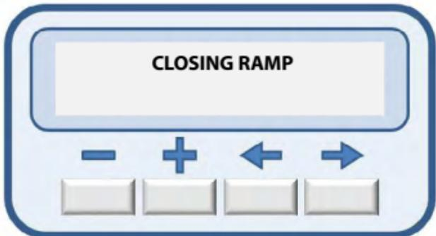
To increase the closing ramp, just press the (+) key, and to reduce it, just press the (-) key.
