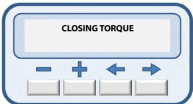
To increase the closing torque, just press the (+) key until the desired torque level and to decrease it, just press the (-) key.
