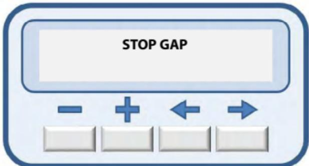
This feature allows encoder motors to establish a gap (space) between the gate leaf and the stop.
