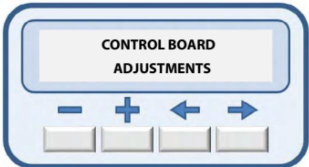
The factory setting is 'allowed'. To lock, press and release the (+) key, and to unlock, press and release the (-) key.
