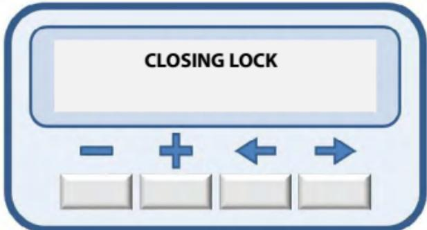
To enable and increase the lock retraction time during the closing path, press the (+) key and to decrease it, press the (-) key.
