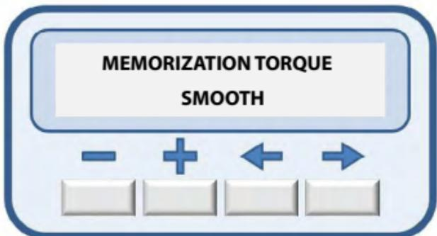
It allows changing the torque memorization of the recorded path. Selecting the soft, moderate or strong options by using the (-) or (+) keys.
