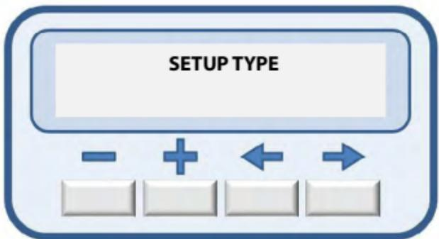
**MODEL:** To select the motor model and the gate model, press and release the (+) or (-) key to choose, then keep the (+) and (-) keys pressed at the same time to start the countdown time from 1 to 5 seconds until the message 'DONE' appears, signaling 'SETUP' is applied.
