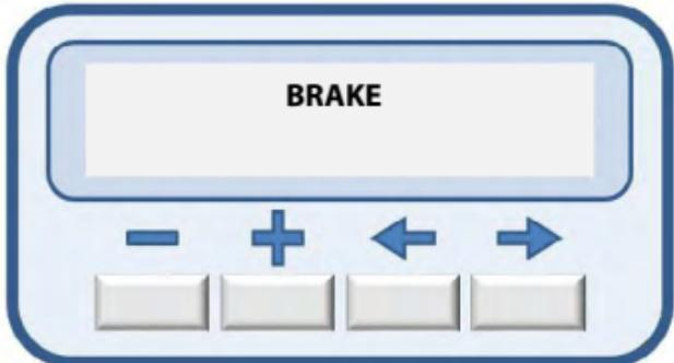
To increase the brake level, just press the (+) key, and to reduce it, just press the (-) key.
