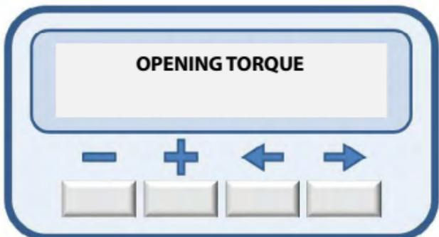
To increase the opening torque, just press the (+) key until the desired torque level and to decrease it, just press the (-) key.
